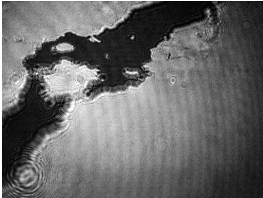
Figure 24**: Film rupture during expansion 510 \times 485 \mu\text{m}^2
