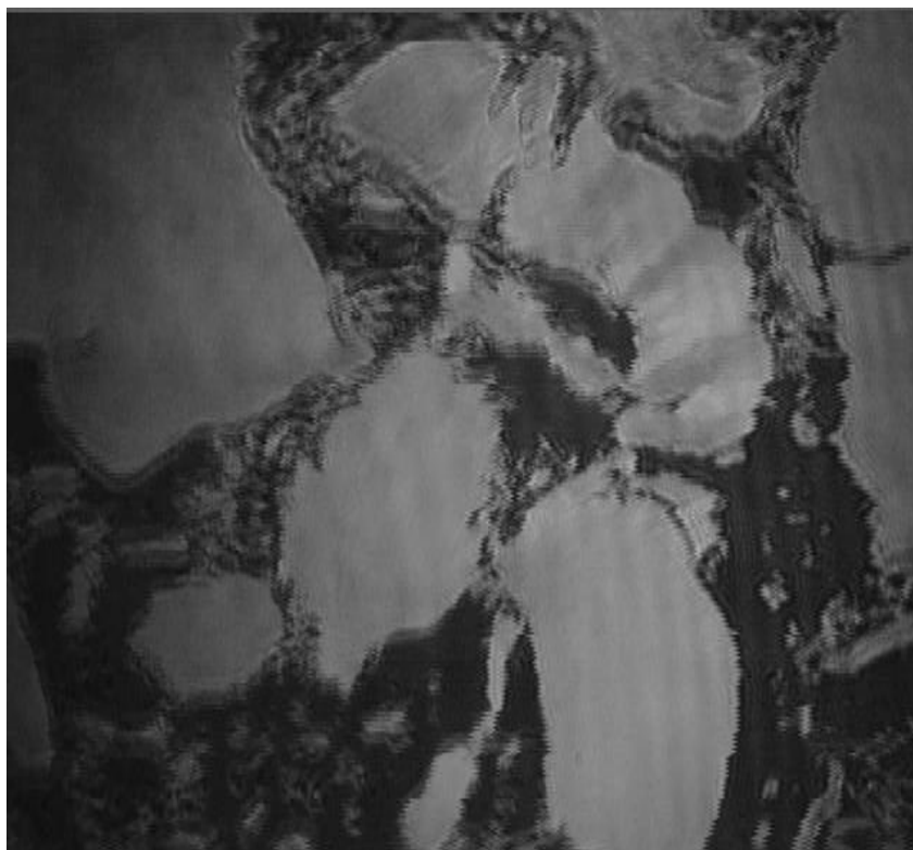
Figure 5*: BAM Image of a Langmuir PBLG film in the gaseous phase, before moving the barriers Image size 510*485 \mu\text{m}^2
