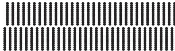
FIG. 3 Structure of a crystal of short-chain molecules like the  $n$ -alkanes. Schematic drawing with two layers. The layer thickness corresponds to the length of the molecules, the distance between neighbours is about  $0.5\ \text{nm}$ .
